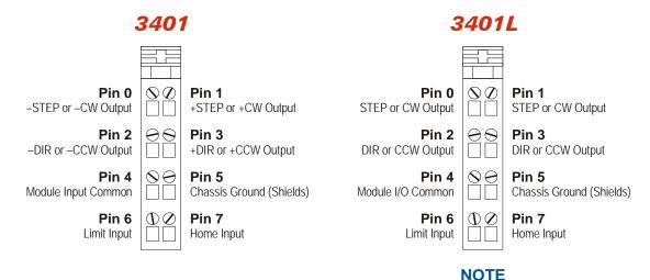
Pins 0 & 1 are electrically connected Pins 2 & 3 are electrically connected You can wire to either pin in these two sets
