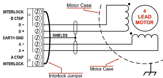
Refer to the torque vs. speed curves on your motor's specifications sheet to determine if you should wire the motor to the SD17040C in series, parallel, or centertap configuration.
