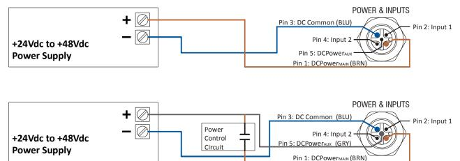
Figure T1.4 M12 Power Wiring
