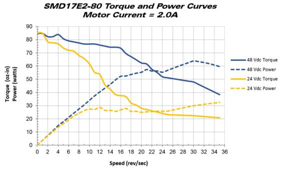
Figure R1.8 SMD17E2-80 Torque and Power Curves
