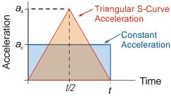
Figure R3.3 Triangular Acceleration
