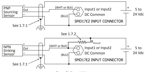
Figure T1.5 Input Wiring
