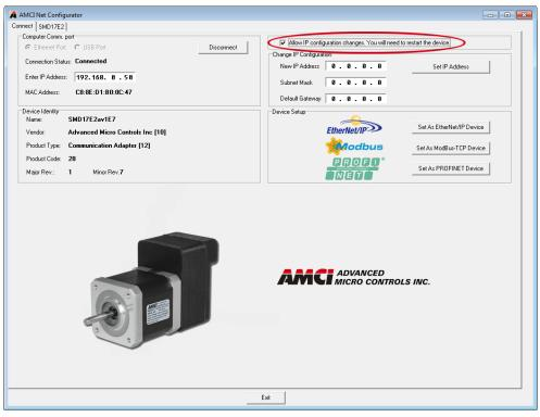
Figure T2.5 Enable IP Address Changes
