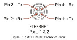
The connector is a standard female four pin D-coded M12 connector that is rated to IP67 when the mate is properly attached.
