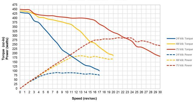
Figure R1.8 SMD34E-450 Torque and Power Curves
