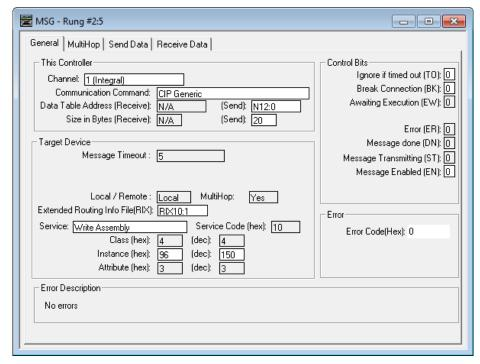
Figure T5.4 Write Message Instruction Setup Screen
