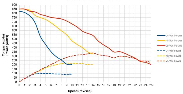
Figure R1.9 SMD34E-850 Torque and Power Curves
