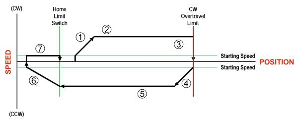
Figure R4.3 Profile with Overtravel Limit
