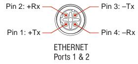
Figure T1.9 M12 Ethernet Connector Pinout
