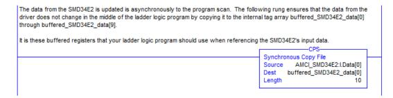
Figure T3.9 Buffer I/O Data
