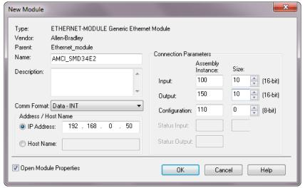
Figure T4.3 Configuration Screen - Generic Device
