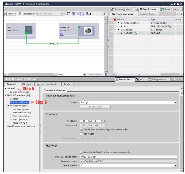
Figure T7.3 Networked Driver IP Addressing
