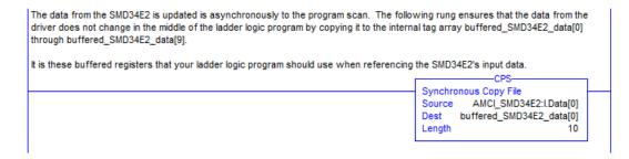
Figure T4.4 Buffer I/O Data
