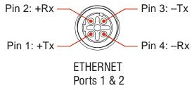
Figure R1.5 Ethernet Connector Pinout
