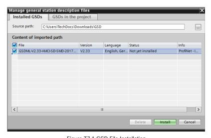
Figure T7.1 GSD File Installation
