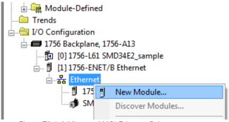
Figure T3.6 Adding an AMCI Ethernet Driver
