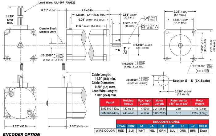
All Encoder signals are 5V differential. (AM26LS31 Line Driver)
