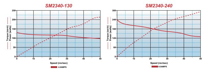
All torque curves generated with SD17040 or SD17060 Stepper Driver
