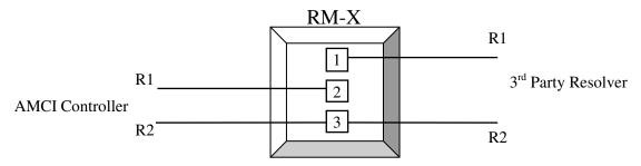
The following diagram shows how to wire the RM-X reference module so that an AMCI resolver will work with a 3<sup>rd</sup> party resolver controller.
