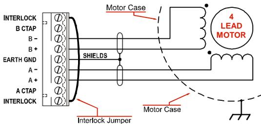
Refer to the torque vs. speed curves on your motor's specifications sheet to determine if you should wire the motor to the SD17060B in series, parallel, or centertap configuration.
