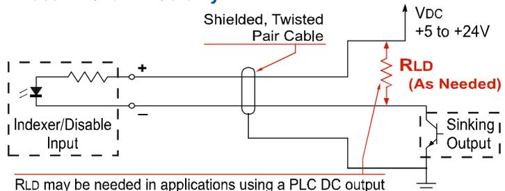
RLD may be needed in applications using a PLC DC output to generate index pulses at high speeds. See the note on this page for more information.
