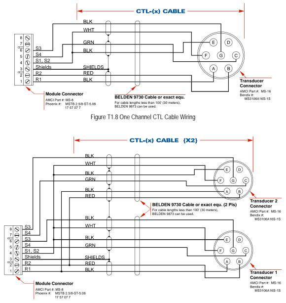
Figure T1.9 Two Channel CTL Cable Wiring
