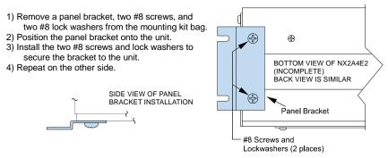
Figure T1.3 Attaching Panel Mount Brackets
