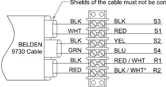
Shields of the cable must not be connected to chassis ground except at the module. Strip the shields back to inside the cable.
