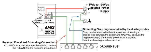
Figure T1.5 Power Supply and Grounding Connections
