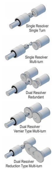
Figure R1.1 Resolver Transducer Types
