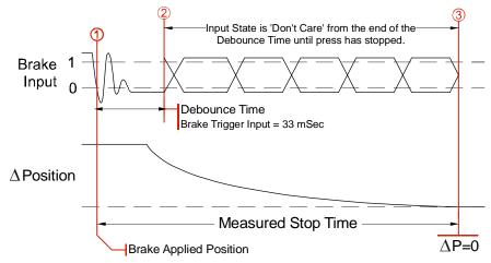
Figure R1.2 below shows how the stopping time is measured.
