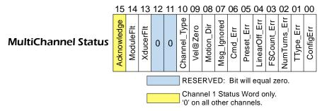
Figure R2.8 Single Resolver Channel Status Word Format
