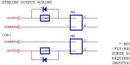
\* NOTE: ANTI-PARALLEL (FLY-BACK) DIODE OR SIMILAR SURGE SUPPRESSION DEVICE IS REQUIRED WHEN SWITCHING INDUCTIVE LOADS
