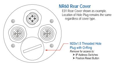
Figure 1.3 Rear Hole Plug Location
