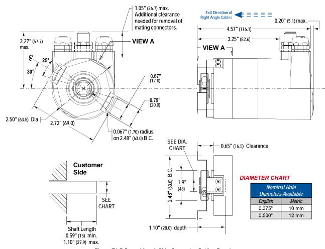
Figure T1.7 Servo Mount, Side Connector Outline Drawing
