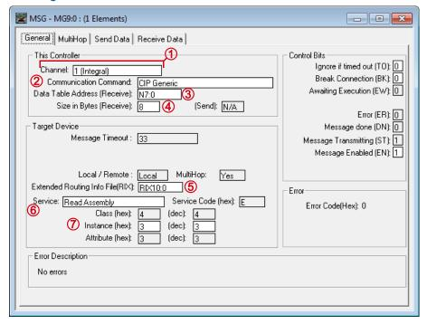
Figure T6.1 RSLogix 500 MSG Example
