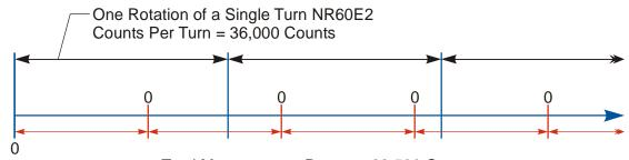
Total Measurement Range = 22,500 Counts NR60 outputs one cycle of counts from 0 to 22,499 for every 225 degrees of rotation.
