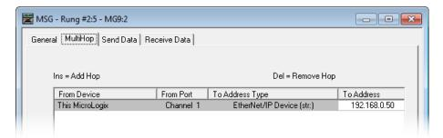
Figure T6.4 MultiHop Address Setting
