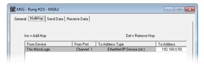
Figure T6.2 MultiHop Address Setting
