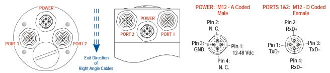
Figure R1.2 Connector Location and Pinout
