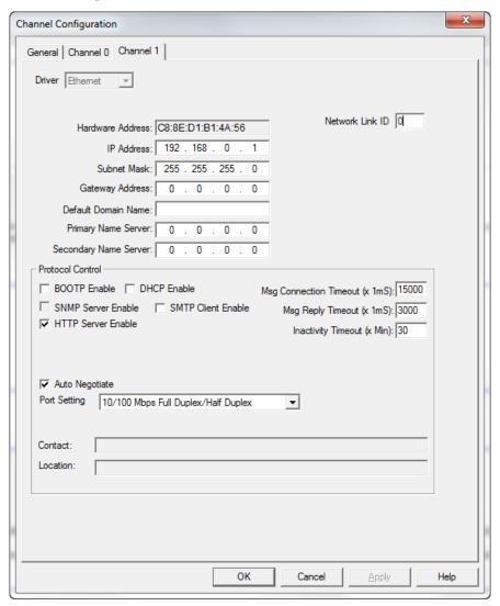
Figure R2.2 MicroLogix Ethernet Configuration Screen
