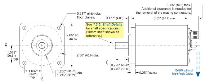
Figure T1.3 Flange Mount, Side Connector Outline Drawing
