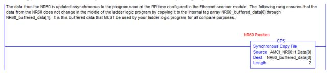
Figure T4.10 Buffer Input Data
