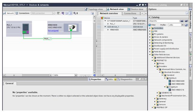
Figure T7.2 NR60E2 added to PROFINET Network
