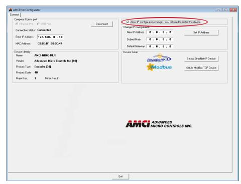
Figure T3.8 Enable IP Address Changes
