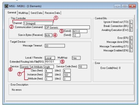
Figure T6.3 RSLogix 500 MSG Example
