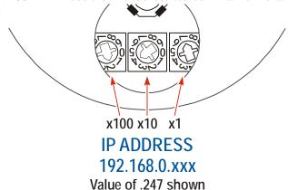
Figure T3.2 Default Setting for IP Address Switches
