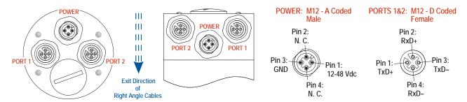
Figure T2.1 NR60E2 Connector Placement
