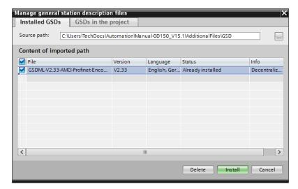
Figure T7.1 GSD File Installation
