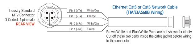
Figure T2.3 MS-28 Sample Wiring
