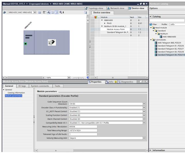
Figure T7.5 Setting NR60E2 Parameters
