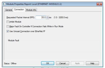
Figure T5.4 Setting the RPI Time
