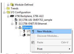
Figure T4.6 Adding an AMCI Ethernet Driver
