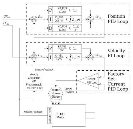
Figure R1.3 Cascade PID Loop Control
