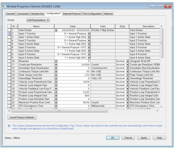
Figure T3.8 SV Servo Configuration with EDS File
