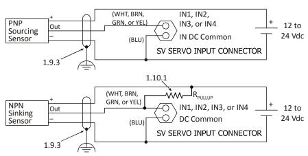
Figure T1.10 Wiring - Digital Inputs 1 through 4
