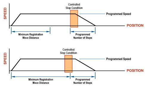
Figure R2.7 Min. Registration Move Distance
