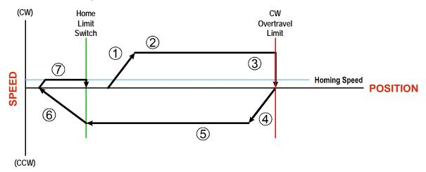
Figure R4.2 Profile with Overtravel Limit
