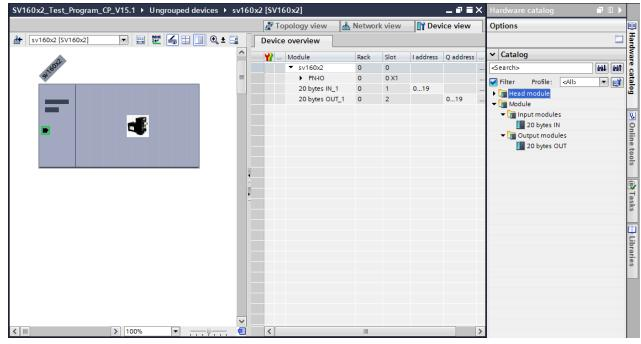
Figure T6.5 I/O Byte Mapping
