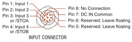
Figure T1.7 Digital Input Connector
