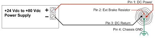
Figure T1.6 M12 Power Wiring
