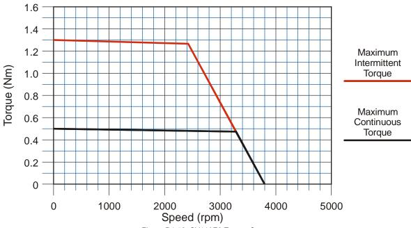
Figure R1.12 SV160E2 Torque Curves
