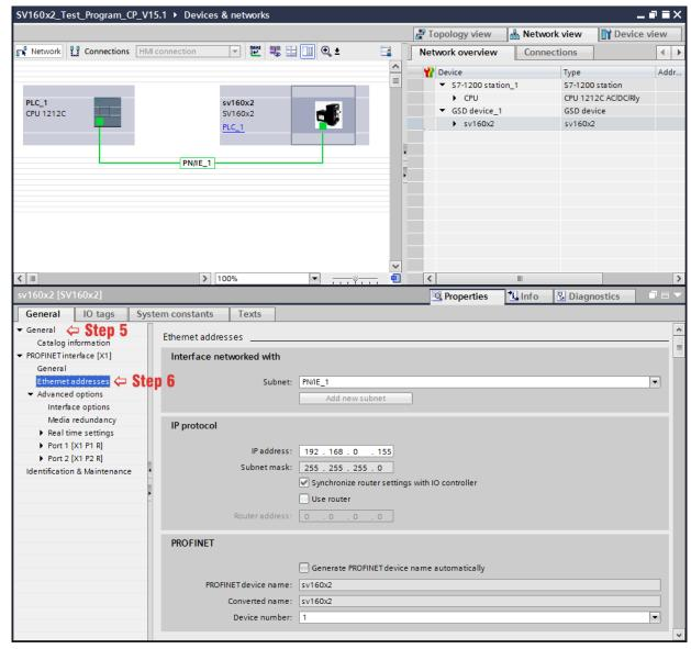
Figure T6.3 SV Servo IP Addressing
