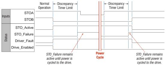
STO Failure occurs whenever the STOA and STOB inputs are in different states for longer than the programmed value of the Discrepancy Timer Limit.
