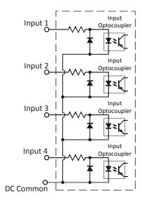
Figure T1.9 Schematic - Inputs 1 - 4
