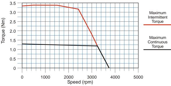
Figure R1.13 SV400E2 Torque Curves
