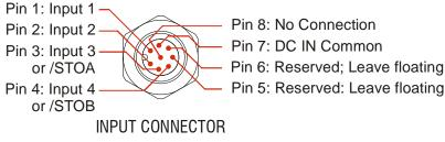
Figure R1.9 M12 Input Connector
