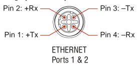
Figure R1.8 Ethernet Connector Pinout
