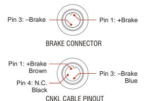
Figure T1.12 M12 Brake Connector Pinout
