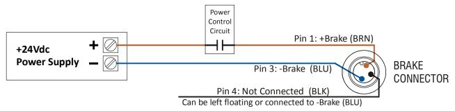
Figure T1.13 Brake Input Wiring
