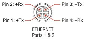
Figure T1.14 M12 Ethernet Connector Pinout
