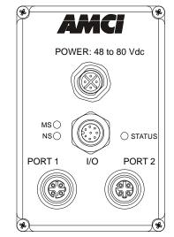
Figure R1.7 SV Servo Connector Locations
