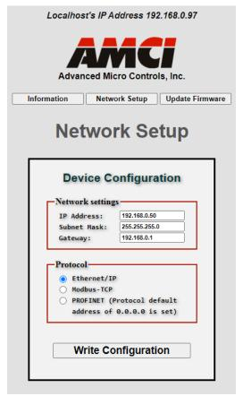
Figure T2.2 SV Servo Network Setup Web Page
