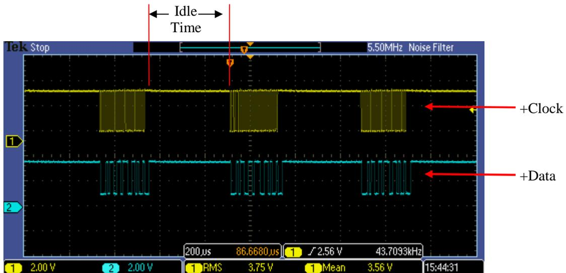
The following image shows three data read cycles of the -Clock and -Data signals. Please note that both the -Clock and -Data signals will be low during the Idle Time.
