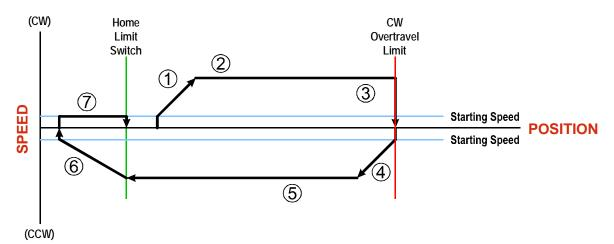
Figure R4.3 Profile with Overtravel Limit
