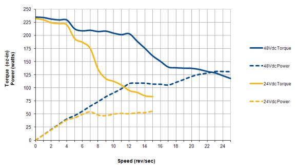
Figure R1.8 SMD23E2-240 Torque and Power Curves
