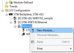
Figure T3.6 Adding an AMCI Ethernet Driver
