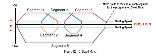
**NOTE** (1) You do not have to preset the position or home the machine before you using a Dwell Move. Because the Dwell Move is based on Relative Moves, it can be run from any location.
