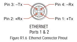
The connector is a standard four pin D-coded female M12 connector that is rated to IP67 when the mate is properly installed.
