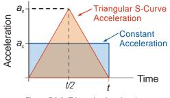
Figure R3.3 Triangular Acceleration
