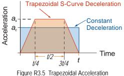
Speed is equal to acceleration multiplied by the time it is applied. This is shown graphically in figure R3.5 as the area of the blue rectangle. In order for the Trapezoidal S-curve acceleration to reach the same speed in the same amount of time, the area of the polygon must equal the area of the rectangle.
