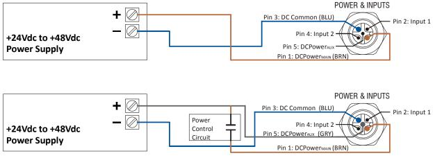
Figure T1.4 M12 Power Wiring
