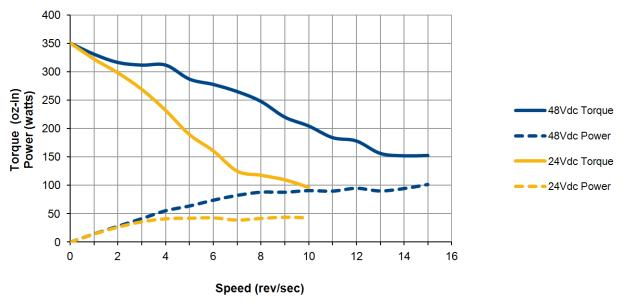
SMD24E2-350 Torque and Power Curves Motor Current = 3.4A
