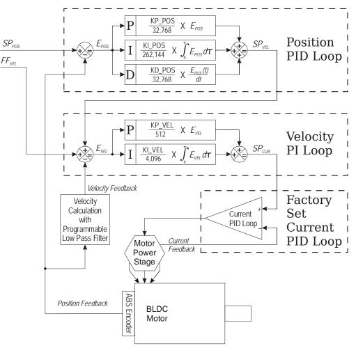
Figure R1.2 Cascade PID Loop Control
