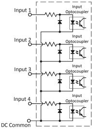
Figure T1.6 Schematic - Inputs 1 - 4
