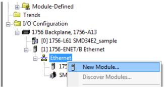
Figure T3.6 Adding an AMCI Ethernet Driver
