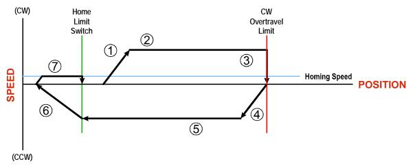
Figure R4.2 Profile with Overtravel Limit
