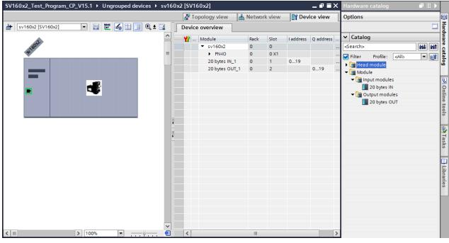
Figure T6.5 I/O Byte Mapping
