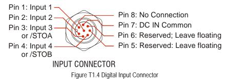
All four digital inputs are single ended, sinking inputs that share a common DC reference, (Pin 7, DC IN Common).
