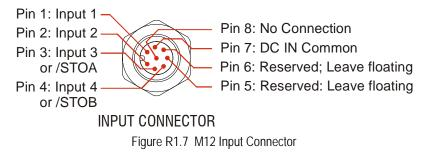
All four digital inputs are single ended, sinking inputs that share a common DC reference. (Pin 7, DC IN Common) All of the inputs accept a nominal 12 Vdc to 24 Vdc signal without the need of a current limiting resistor. Additional information on how the digital inputs can be used can be found in the *Available Discrete Inputs* section of the chapter, starting on page 16.
