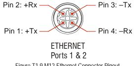
Figure T1.9 M12 Ethernet Connector Pinout
