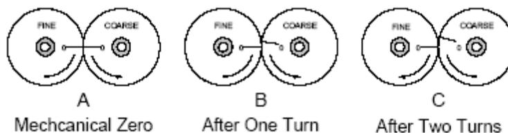
The fine resolver yields the absolute position within the turn directly. Using a proprietary algorithm, the electronic module determines the number of turns completed by the difference in positions of the two resolvers. The absolute multi-turn position is then calculated as ((number of turns completed \* counts per turn) + fine resolver position).
