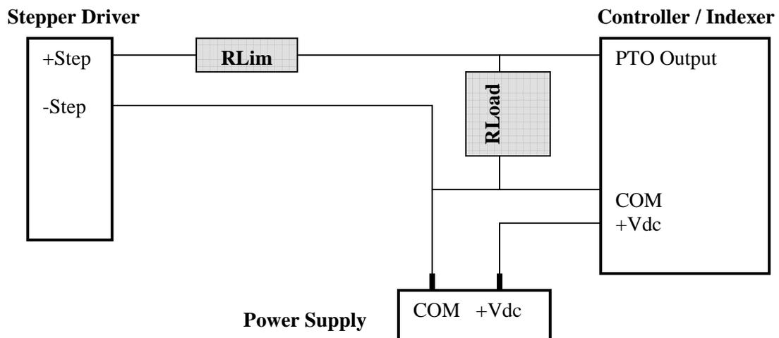
The value of current limiting resistor R<sub>Lim</sub> shown in the above diagram will vary with the Power Supply used to power the PTO output. The following table shows the possible values of this R<sub>Lim</sub> resistor.
