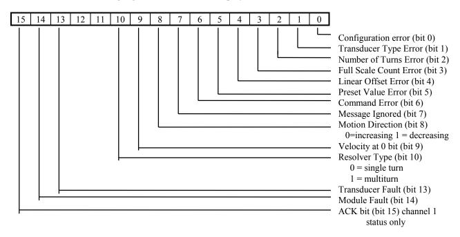
Configuration Error: Set if any of the unused bits in the configuration word are set
