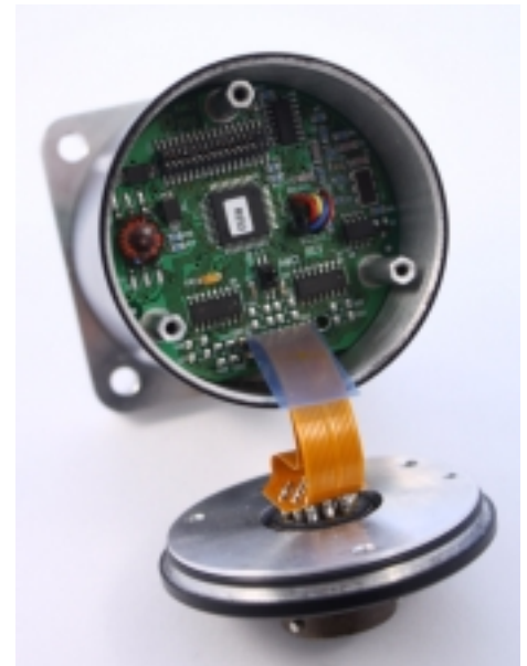
Figure 2.1 DuraCoder with Cover Removed
