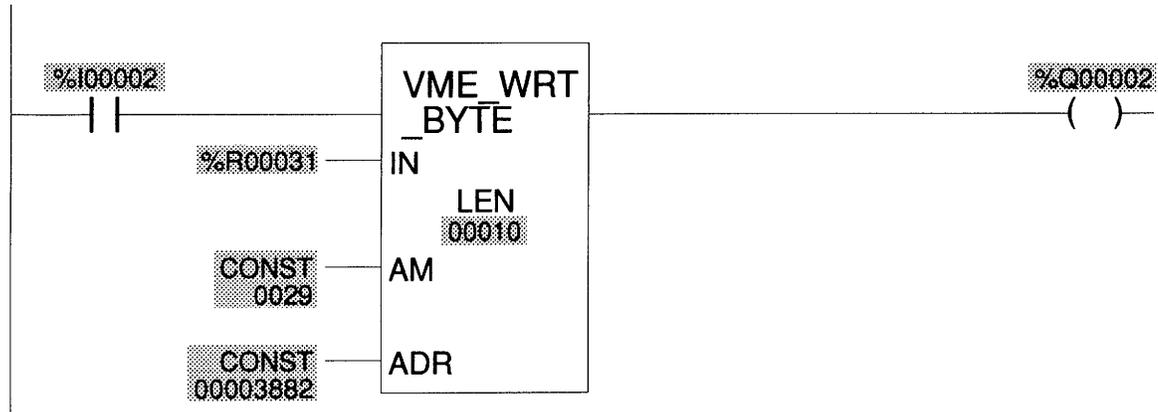
Fig 7.1 GE Fanucs' VME\_WRITE\_BYTE Function
