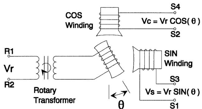
Fig 1.2 Resolver Schematic
