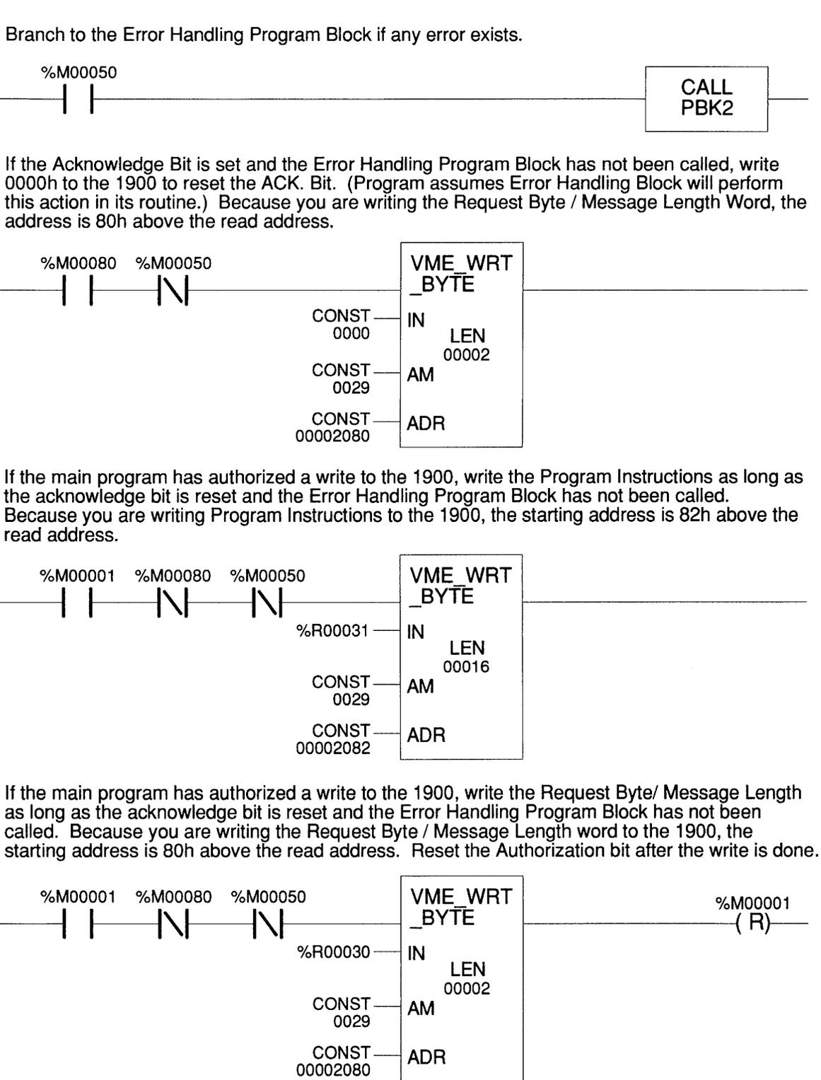
Fig 7.6 Sample Ladder Logic Program Block
