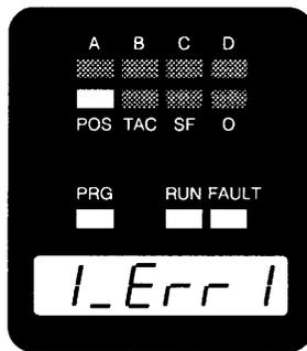
Fig 2.9 Transducer Fault
