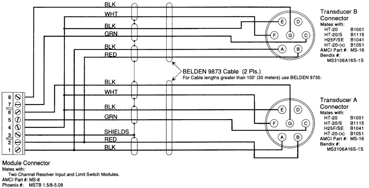
Fig 3.10 C2T-(x) Wiring Diagram
