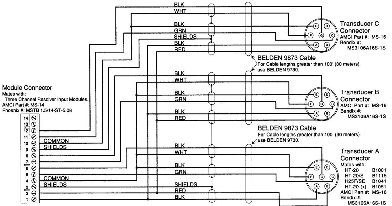
Fig 3.11 C3T-(x) Wiring Diagram
