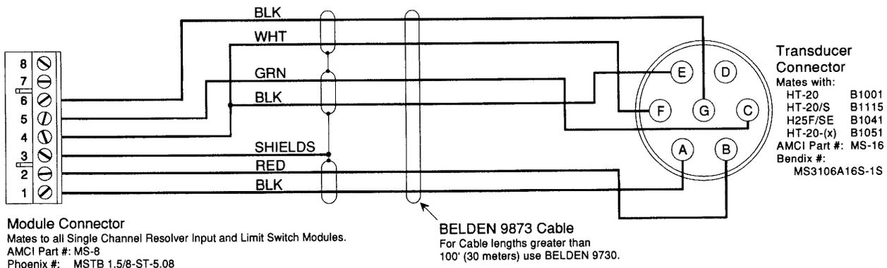
Fig 3.9 C1T-(x) Wiring Diagram
