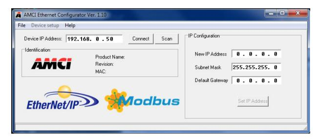
2. The NX3A1E2-M units ship with a default IP address of 192.168.0.50.
