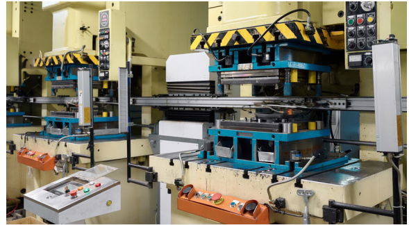
Heavy stamping and metal forming equipment often requires resolver-based feedback because of vibration, shock loading, and electrically noisy operating conditions.
