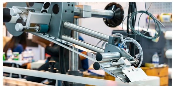
Labeling systems are a common example of applications requiring simple, single-axis positioning rather than a full multi-axis motion platform.
