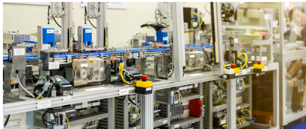
Compact automation equipment often leaves little room for additional rack-based expansion. Distributed Ethernet modules can be mounted near the machine, reducing cabinet redesign and simplifying installation.
