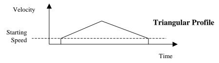
Regardless of the type of Velocity Profile that is being run, the following equations can be used to determine both the time to accelerate and the number of steps needed to accelerate. These formulas can also be used to calculate the time and distance to decelerate.
