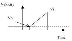
The acceleration rate entered in these equations <u>must</u> have units of steps/second/second, not the steps/ms/second used by the NX1F4X module. See the Calculation Notes below for a complete explanation.
