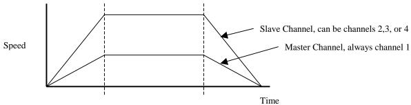
While being the Master, Channel 1 can run any type of move profile.
