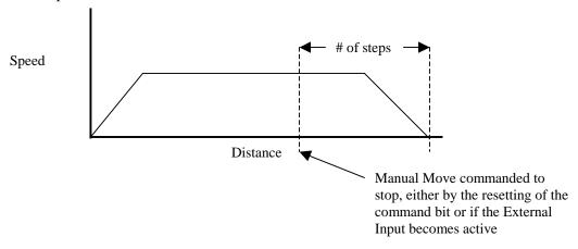
When performing a Registration Move, the following conditions will set the *Command Error bit* (Status Word 1, bit 12).
