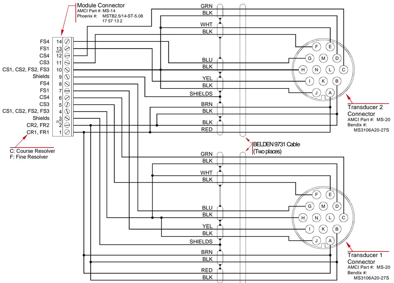
**Note:** Pin 1 of the Transducer Input Connector is towards the bottom of the module when plugged in.
