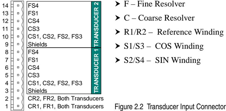
Figure 2.2 Transducer Input Connector
