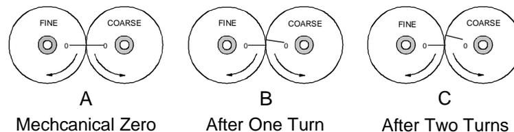
Figure 1.2 Resolver Alignment in Multi-turn Transducers
