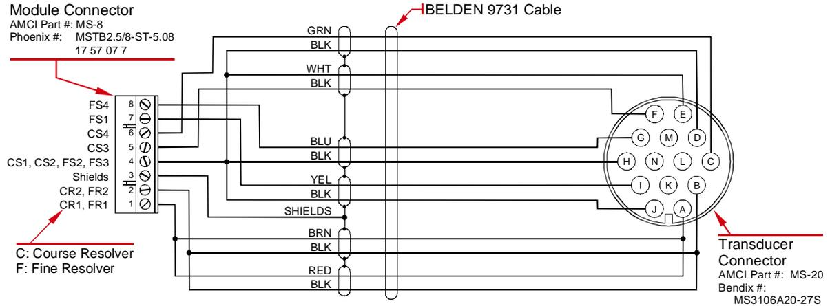
**Note:** Pin 1 of the Transducer Input Connector is towards the bottom of the module when plugged in.
