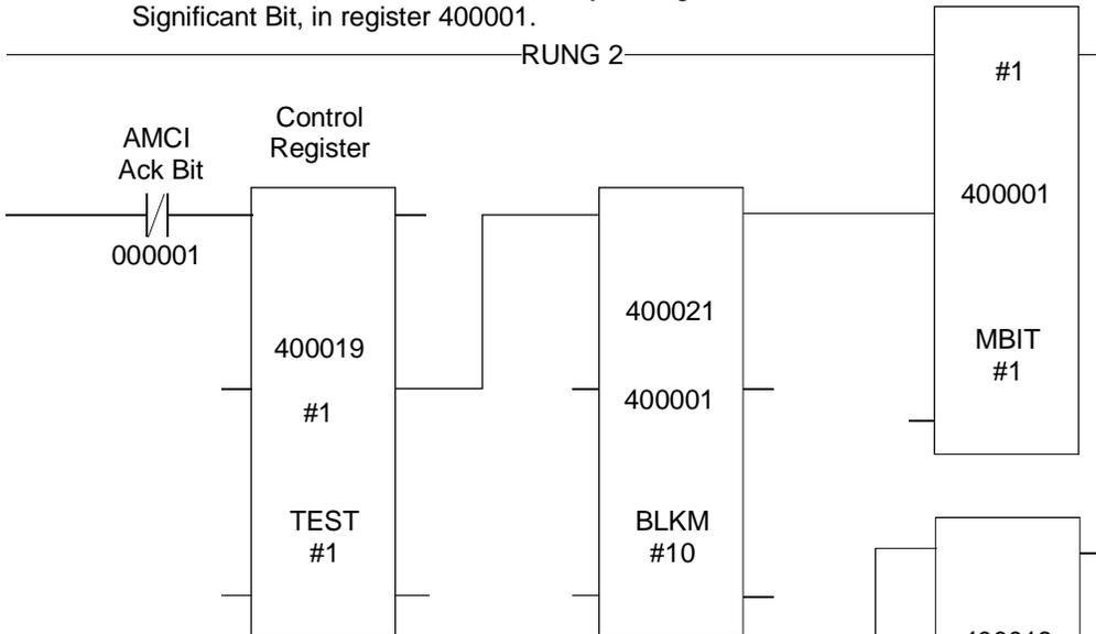
RUNG 3 When Acknowledge Bit 000001 is set, the 1860Q module has accepted the data transferred to it by the previous rung. When the transfer is complete, this rung resets register 400019, which initiated the programming cycle to 0. The programming cycle is now complete.
