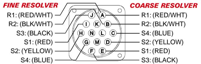
Figure 2.3 Transducer Connector Pin Designations
