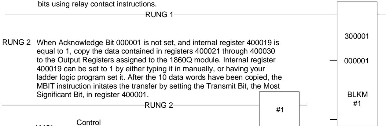
RUNG 2 When Acknowledge Bit 000001 is not set, and internal register 400019 is equal to 1, copy the data contained in registers 400021 through 400030 to the Output Registers assigned to the 1860Q module. Internal register 400019 can be set to 1 by either typing it in manually, or having your ladder logic program set it. After the 10 data words have been copied, the MBIT instruction initiates the transfer by setting the Transmit Bit, the Most Significant Bit, in register 400001.
