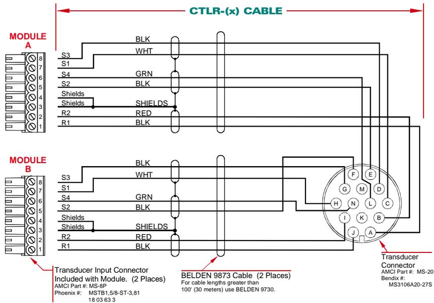
Figure 6.2 CTLR(x) Wiring Diagram
