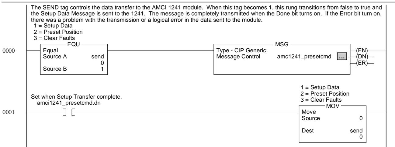
Figure 3.3 System Checkout Ladder Logic
