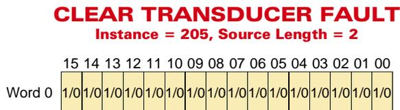
Figure 4.8 Clear Transducer Fault Format
