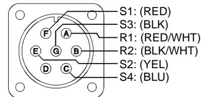
Figure 4.12 Transducer Connector Pinout
