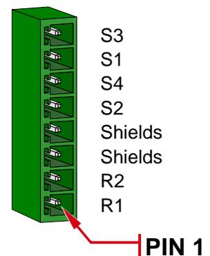
Figure 4.3 Transducer Input Connector
