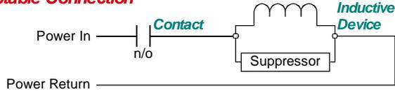
The acceptable connection suppresses noise at its source. The wiring that connects the load to the power supply and contacts will not radiate noise when the load is switched and noise will not be coupled into the power supply.
