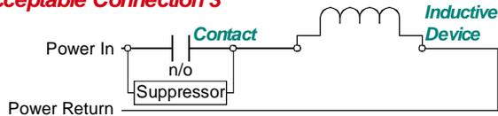
This connection protects the contact but nothing else. Noise can radiate through the load's wiring where it can be coupled into other cables or into the power supply. Noise in the supply may affect any device powered by it, including the Control-Logix system. Also, if the suppressor shorts out, the load will always receive power.
