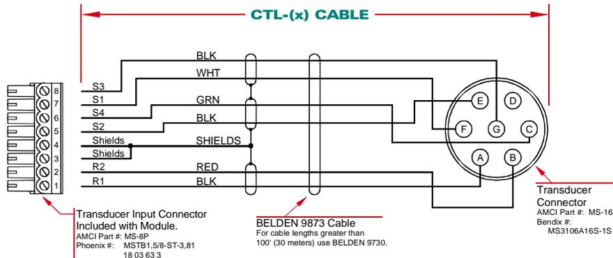
Figure 3.2 CTL-(x) Wiring
