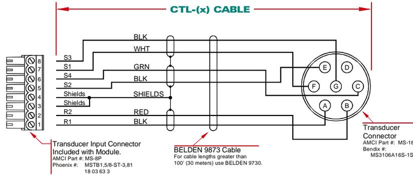
Figure 4.10 CTL-(x) Wiring Diagram
