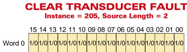
Figure 8.4 Clear Transducer Fault Data Format
