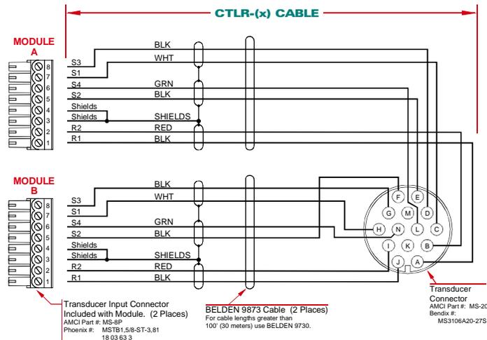
Figure 4.11 CTLR-(x) Wiring Diagram
