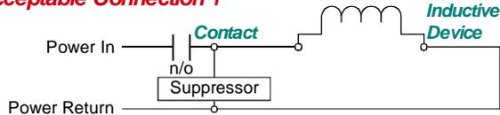
This connection protects the power supply and contact, but allows noise to radiate through the load's wiring where it can be coupled into other cables around it, including the 1241's transducer cable.
