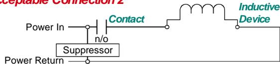
This connection protects the power supply but nothing else. Noise can radiate through the load's wiring where it can be coupled into other cables around it and the contact may eventually be damaged by high voltage inductive spikes.
