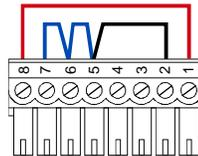
Figure 3.1 Faking a Transducer Connection
