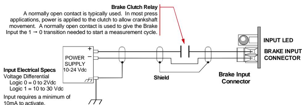
Figure 4.4 Brake Input Wiring
