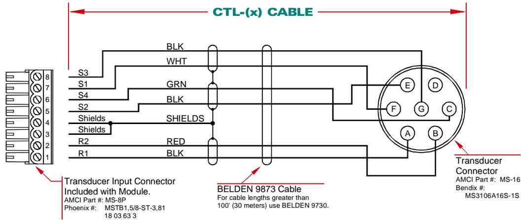
Figure 6.1 CTL(x) Wiring Diagram
