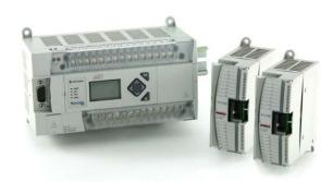
MicroLogix 1100, 1200, and 1400, and are easy to program using Allen-Bradley's RSLogix 500 software.
