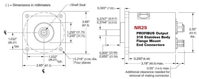
Figure 2.5 Flange Mount, End Connector, Stainless Steel Body Outline Drawing
