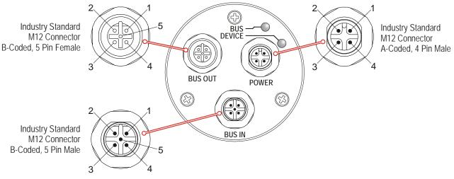
Figure 2.11 Connector Pinout
