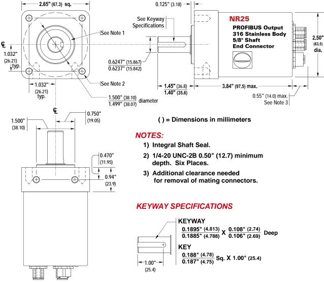
Figure 2.8 5/8" Shaft, Flange Mount, End Connect Outline Drawing
