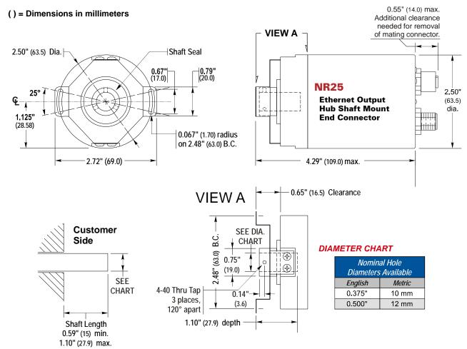
Figure 2.9 Hub Shaft Mount, End Connect Outline Drawing
