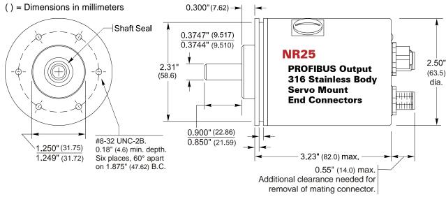
Figure 2.2 Servo Mount, End Connector, SS Body Outline Drawing
