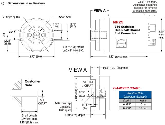
Figure 2.10 Hub Shaft Mount, End Connect Outline Drawing
