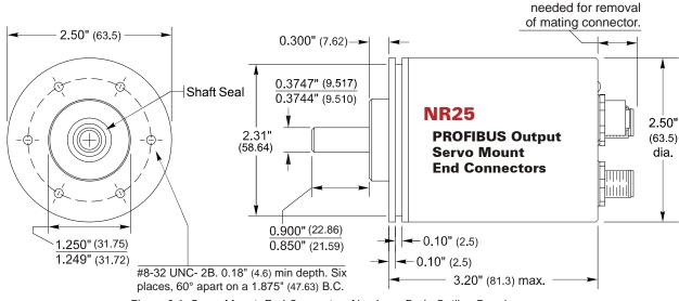
Figure 2.1 Servo Mount, End Connector, Aluminum Body Outline Drawing
